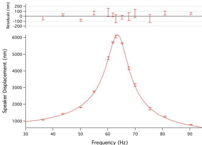
Fig. 3. Frequency response curve for the loudspeaker with corresponding residuals plot. The data were fitted to the equation for a driven, damped, harmonic oscillator.
