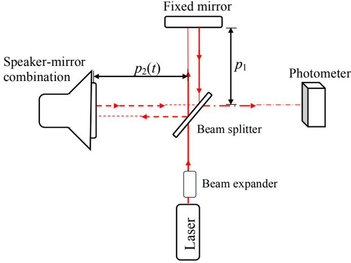
Fig. 1. Experimental setup, illustrating the Michelson interferometer and the paths of its arm lengths  $p_{1,2}$ . The He-Ne laser travels through a beam expander onto a beam splitter where two perpendicular waves propagate towards respective mirrors. They recombine and their interference pattern is measured by the photometer.
