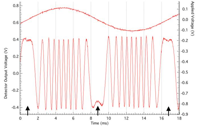
Fig. 2. Typical figure observed on the oscilloscope screen for  $f = 62.98$  Hz and  $V_0 = 100$  mV, as recorded by a LabView program. The curve shows the AC component of the detector output voltage. Each complete cycle of the curve corresponds to a speaker cone displacement of  $\lambda/2$ , with each arrow corresponding to a turnaround point.
